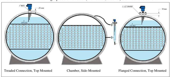
Depending on what levels are determined for switching signals, Probe tips must be cut to desired lengths before being connected to the body.
